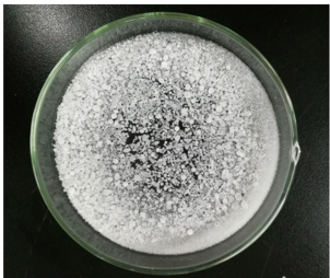
图 1 甲基丙烯酸甲酯的悬浮聚合产物 Figure 1 Product of poly methyl methacrylate prepared by suspension polymerization method
